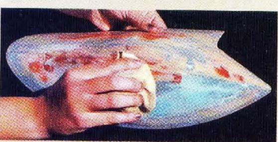
Liberally apply at least four coats of paste wax to the plugs before you add the fiber-glass cloth and resin.
