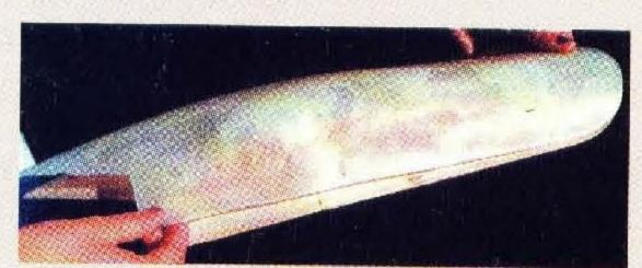
After all the resin has cured, you can remove the part from the plug and trim it to shape. Use the plug's shape as a guide.
